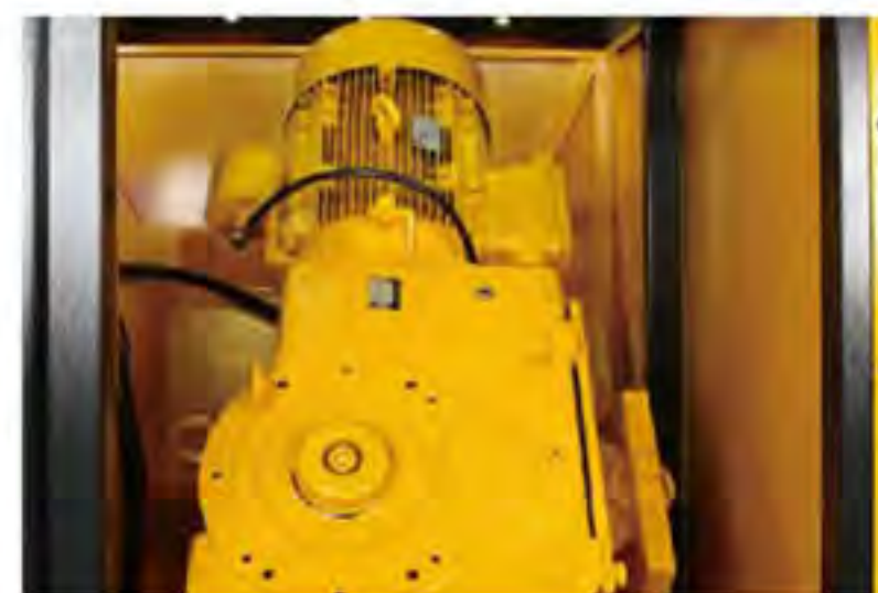
High torque Gearbox quietly powers the saw blade.
