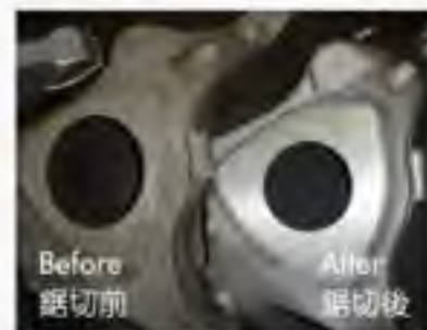
轉向器零件冒口鋸切 Sprue of steering parts cutting
